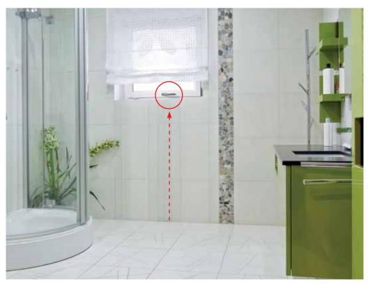
When the window handle is turned through 180 degrees, the interconnected locking mechanism mechanically transmits the tilt or close instruction to the scissor-stay arm of the comfort scissor stay.
