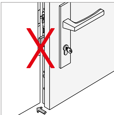
Do not lock the locking bar when the door is open!
