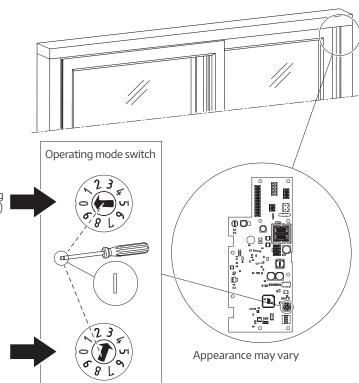
A factory reset (Full Init) with complete initialisation must be performed after adjusting the operating mode switch.
