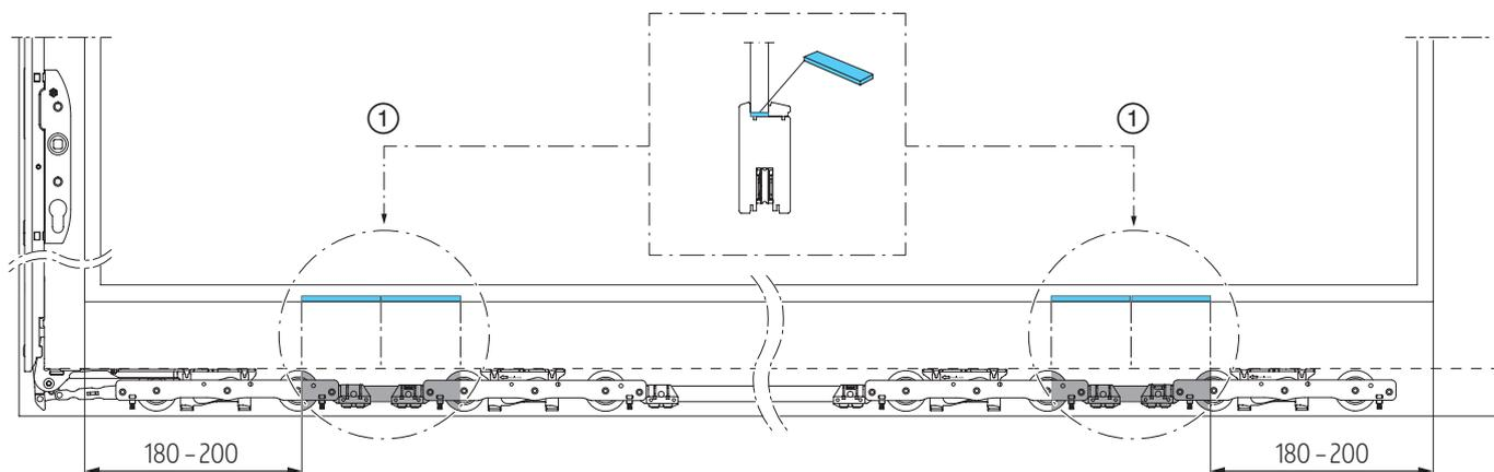
**Abb. 2:** Move HS 500 Nut 22 x 42; (vier Tragklötze)
