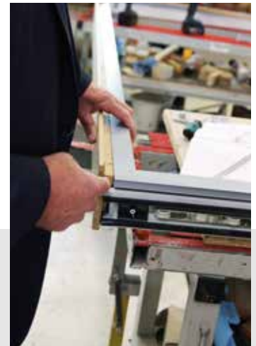
The timber frame is applied
