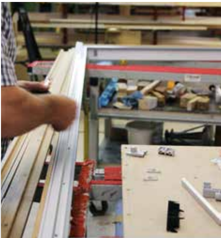
The sealing rail is attached
