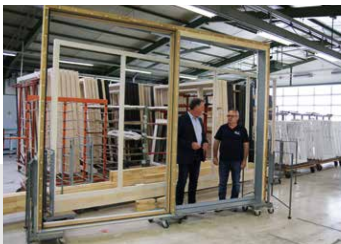
Almost finished sash. On the outside, the aluminium frame is clipped on. Here, you can see how the sash frame disappears into the frame on the right and the glass lights become the passage lights.
